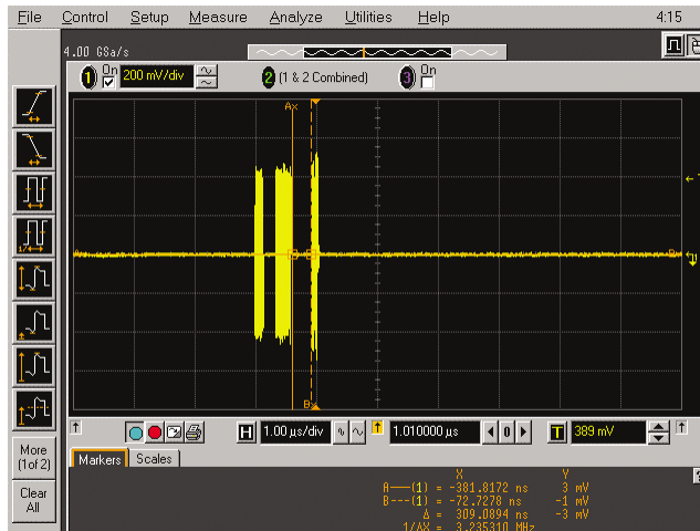
Figure 13. Device inter-packet gap.
